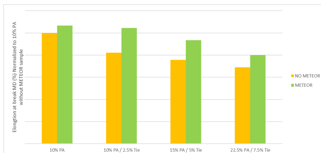
Figure 4. Elongation at break of PE/PA blends in machine direction, with and without METEOR (normalized to PE/PA blend at 10% without METEOR).
