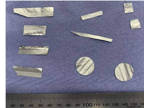
Materials delaminated at 90 °C
