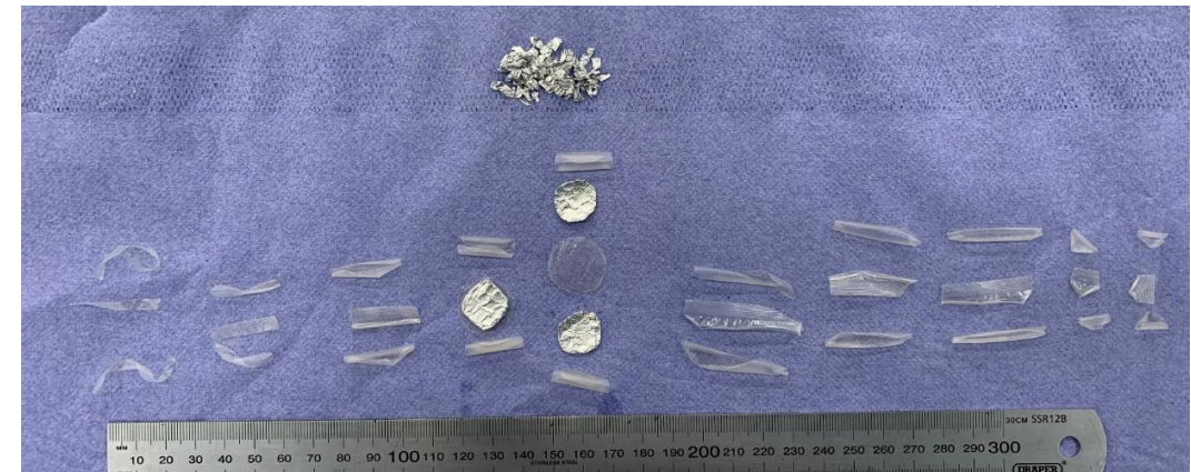
Materials delaminated at 90 °C
