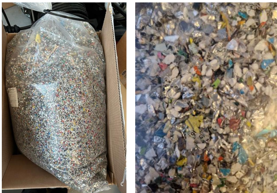
Figure 4 Real metallized film waste sample after pre-treatment by AIMPLAS.
