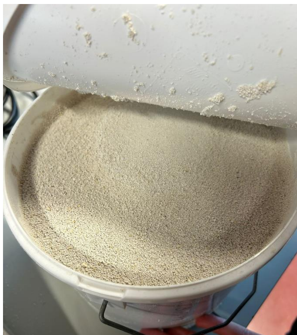
Figure 8 Polyolefin product recovered from the CIMPA TRL5 pilot.
