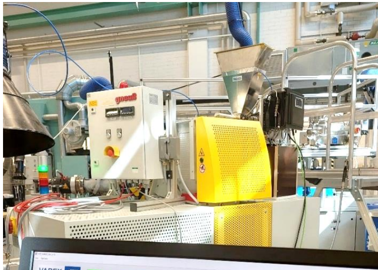
Feeding of multi-layer plastic film waste
